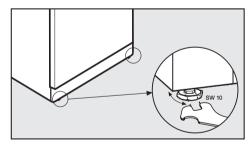
■ To align the appliance, adjust the feet using a suitable spanner.
